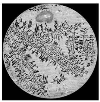
Dendrite formations, above, affect the process of metals casting. Results from this International Space Station investigation are an example of materials science data that would be included in the MaterialsLab database.
