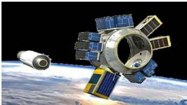
Based on the EELV Secondary Payload Adapter (ESPA) it provides a facility to deploy multiple small satellites to a variety of orbits including low-Earth, geostationary as well as Earth-Sun Lagrange points orbits and lunar orbits.
